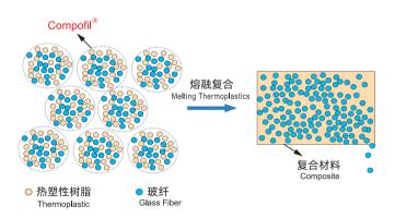
Direct roving, good compatibility with resins, excellent mechanical properties of composite products
